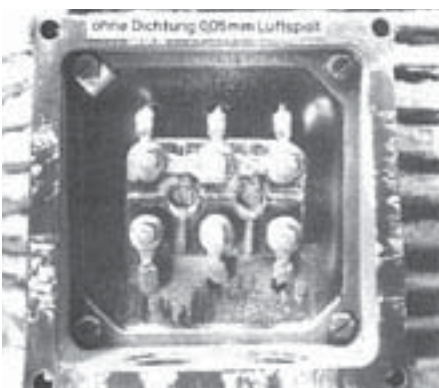
Figure 10: Test result with the gap reduced to 0.05 mm, test period approx. 200 minutes
